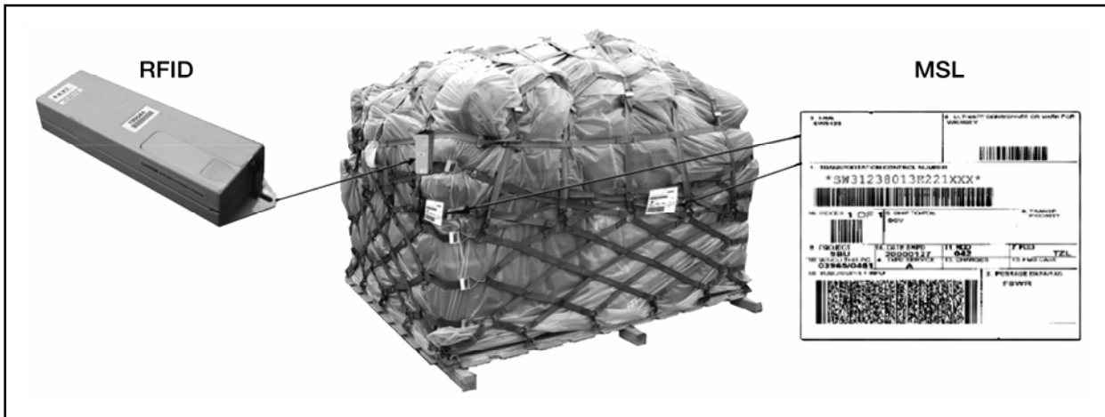
Figure D-5. Pallet Marking
